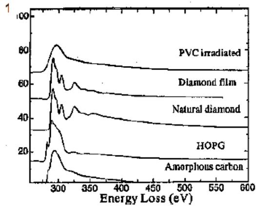
Figure 1. Extended fine structure in the transmission mode
