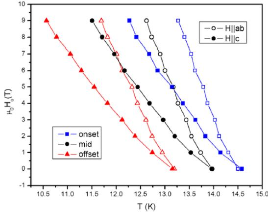
FIG. 2.  $H_{c2}$  critical field versus temperature (H-T phase diagrams) determined for conditions  $R = 0.9R_n$ , (onset),  $R = 0.5R_n$ , (mid) and  $R = 0.1R_n$ , (offset) where  $R_n$  is the normal state resistance. Full and empty symbols correspond to  $H||c$  and  $H||ab$ , respectively.
