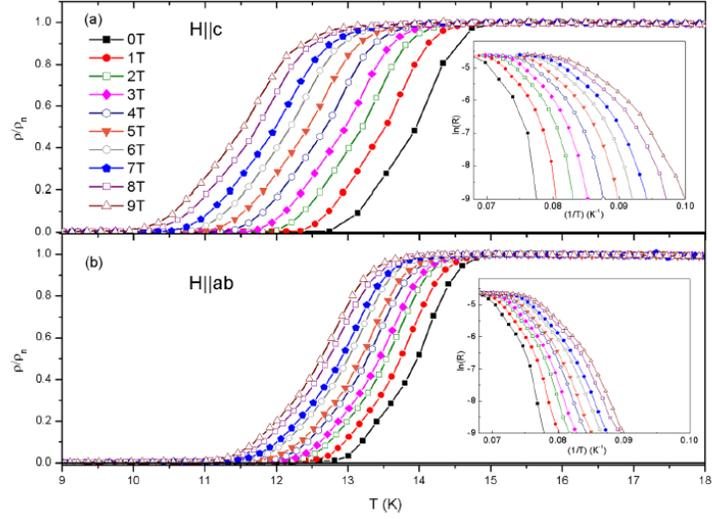
FIG. 1. Resistivity (normalized to the normal state resistivity) versus temperature for magnetic applied magnetic fields of 0, 1, 2, 3, 4, 5, 6, 7, 8, and 9 T. (a)  $H||ab$  and (b)  $H||c$ . Insets: Arrhenius plots for the same applied magnetic fields (a)  $H||ab$  and (b)  $H||c$ .
