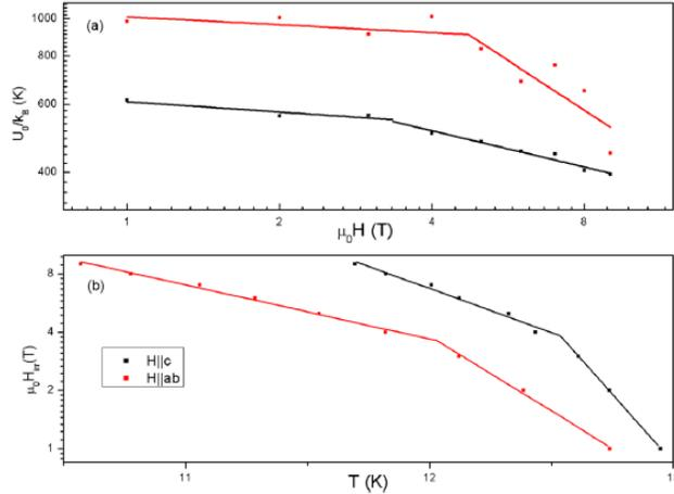
FIG. 3. (a) Activation energy versus applied magnetic field, in the  $H||ab$  and  $H||c$  directions, respectively. (b) Irreversibility line  $\mu_0 H_{irr}$  versus temperature in the  $H||ab$  and  $H||c$  directions, respectively.
