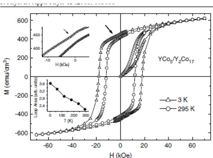
**Figure 2.** Hysteresis loops from  $\text{YCo}_5(70 \text{ wt}\%)/\text{Y}_2\text{Co}_{17}(30 \text{ wt}\%)$  nanocomposite powders measured at 3 and 295 K. The small ‘knee’ in the 3 K data (indicated by the arrow) suggests that the exchange coupling becomes less effective at low temperatures. The lower inset shows the temperature dependence of the area closed by the  $M(H)$  curves.
