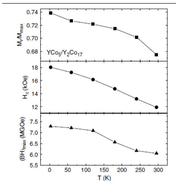
**Figure 1.** Coercivity, squareness and maximum energy product as a function of temperature for  $\text{YCo}_5$ (70%)/ $\text{Y}_2\text{Co}_{17}$ (30%) annealed at 1073 K for 1.5 min.
