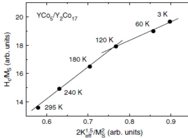
**Figure 4.**  $H_C/M_S$  versus  $2K_{\text{eff}}^{1.5}/M_S^2$  for temperatures between 3 and 295 K. The two solid lines are linear fits to the data within the 3–120 K and the 120–295 K temperature intervals.
