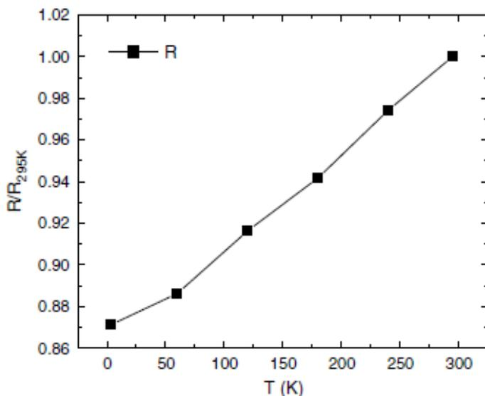
**Figure 3.** Temperature dependence of the exchange-coupled volume ratio  $R$  normalized to its room-temperature value.
