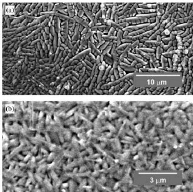
Fig. 2. SEM micrograph of longitudinal plane surface of the ribbon obtained with: (a) 25m/s Cu roll velocity; (b) 48.5m/s Cu roll velocity.
