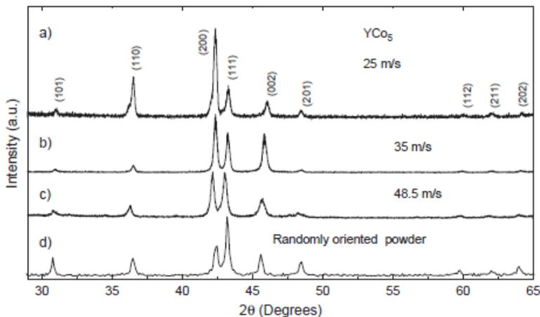
Fig. 1. X-ray diffraction patterns of the melt-spun ribbons obtained with different Cu roll velocities and a randomly oriented powder sample.
