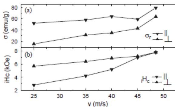
Fig. 4. (a) Remanence magnetization and (b) coercivity dependence with the Cu roll velocity and the applied field direction.
