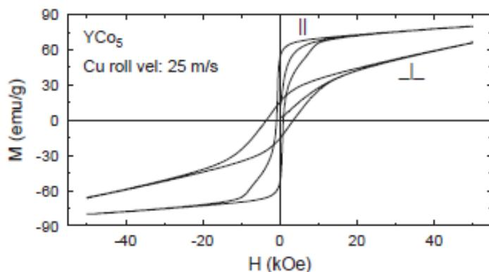
Fig. 3. Hysteresis loops measured with the magnetic field applied parallel and perpendicular to the plane of a ribbon melt-spun with  $v = 25\text{m/s}$ .
