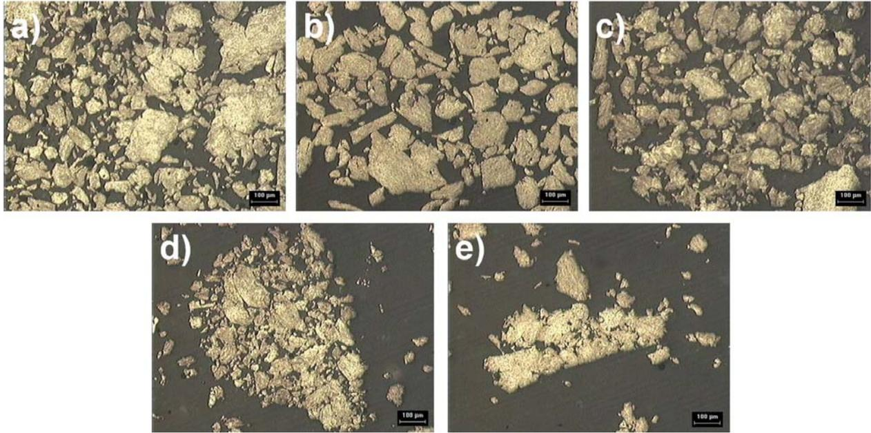
**Figure 2.** Powder morphology evolution of the  $Al_{7075}$ -Ag-C NP nanocomposites as a function of silver nanoparticles content, with 5 h of milling: a) 0.0, b) 0.5, c) 1.0, d) 1.5 and e) 2.0 wt.% of Ag-C NP.
