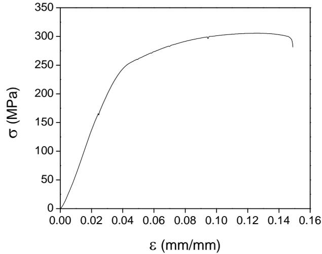
**Figure 5.** Stress–strain curve of the Al<sub>7075</sub> alloy milled for 5 h and tested in the extrusion direction.
