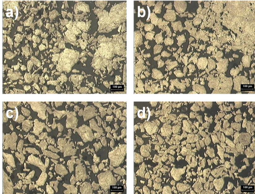
**Figure 1.** Powder morphology evolution of the  $Al_{7075}$  alloy as a function of the milling time: a) 5h, b) 10h, c) 15h and d) 20 h.
