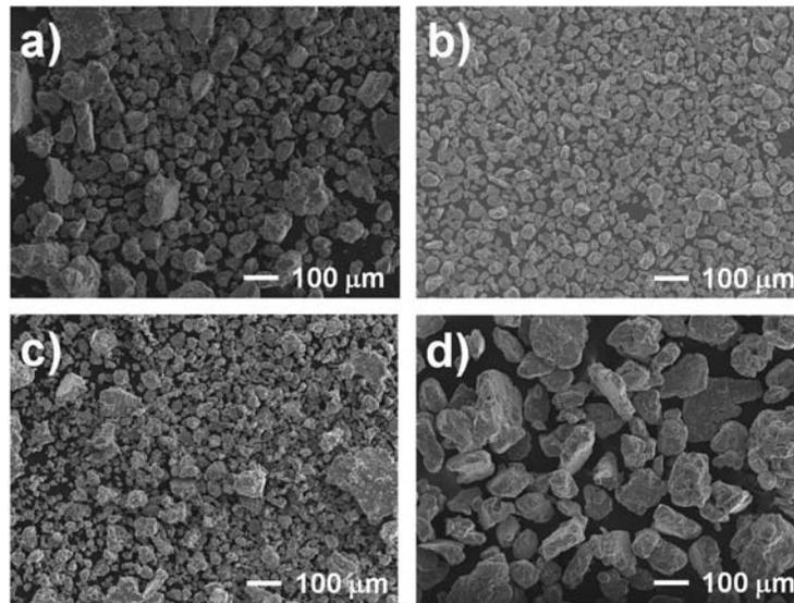
**Figure 3.** Powder morphology evolution of the  $Al_{7075}$ -Ag-C NP nanocomposites after MM with: a) 5h and 2.0 wt.%, b) 10 h and 2.0 wt.%, c) 15 h and 2.0 wt.%, and d) 20 h and 0.0 wt.% of Ag-C NP.
