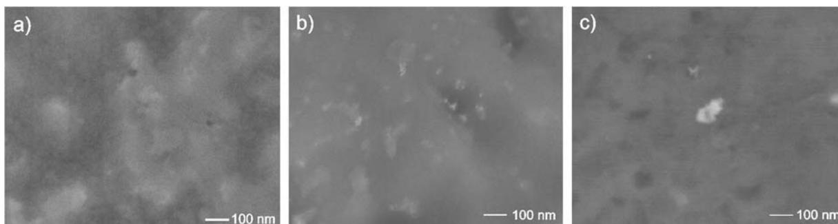
**Figure 4.** Morphological evolution of the extruded  $Al_{7075}$ -Ag-C NP nanocomposite after a) 10 h and 0.0 wt.% of Ag-C NP, b) 10 h and 1.5 wt.% of Ag-C NP, and c) 10 h and 2.0 wt.% of Ag-C NP.
