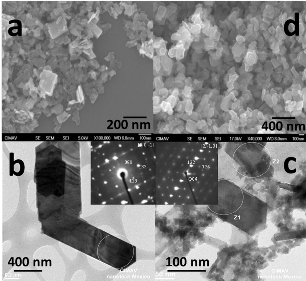
Fig. 1: FIG. 1 SEM, TEM and SAED images of  $W_{1-x}Mo_xO_3 \cdot 0.33H_2O$  ( $x = 0, 0.25, 0.50, 0.75$ ) nano/microstructures
