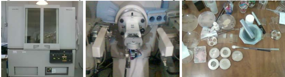
Figure 4. Images of X-ray Diffractometer and sample preparation.
