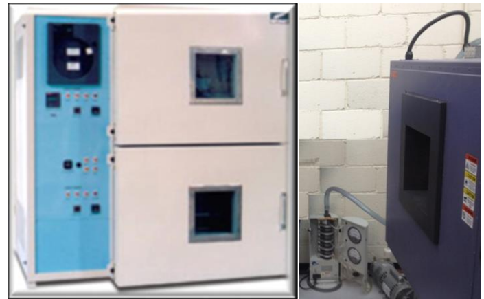
Fig. 1 Thermal Shock Chamber Associated Environmental Systems AES SM-2105D, coupled with MOUDI.
