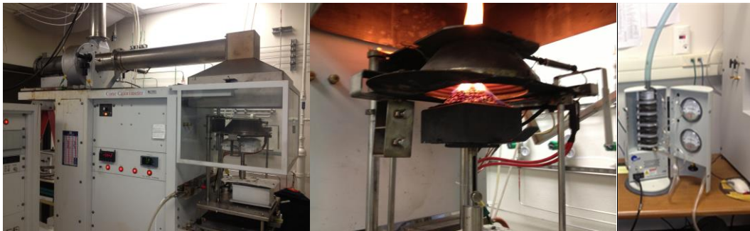
Fig.3 Fire Testing Technology cone calorimeter in operation coupled to MOUDI-110
