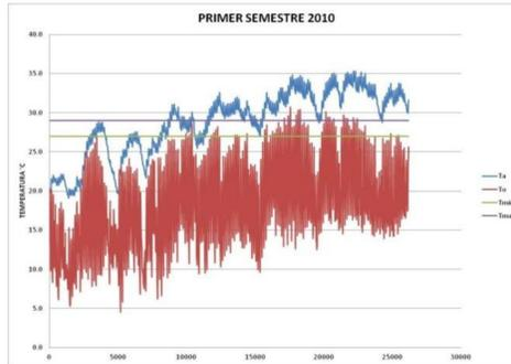
Behavior of the water temperature for the first semester of 2010 with a collector area of 338m<sup>2</sup> and 195 collectors
