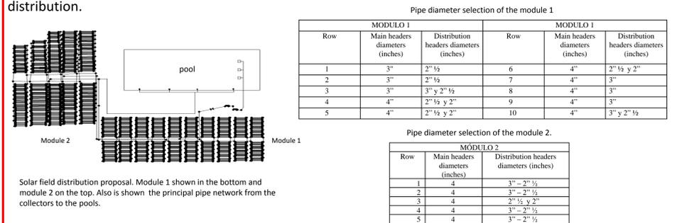
Solar field distribution proposal. Module 1 shown in the bottom and module 2 on the top. Also is shown the principal pipe network from the collectors to the pools.
