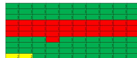
Flow distribution in module 1. The red ones corresponds to an irrigation >11 L/min. Green ones are into the optimum irrigation. The yellow ones are below 3 L/min.
