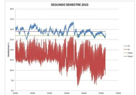
Behavior of the water temperature for the second semester of 2010 with a collector area of 338m<sup>2</sup> and 195 collectors.
