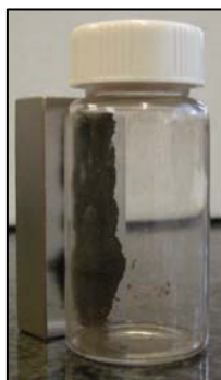
Figure 3: Magnetic behaviour of Mn-Zn Ferrite nanoparticles synthesized with 20% of dispersed phase in O/W microemulsion
