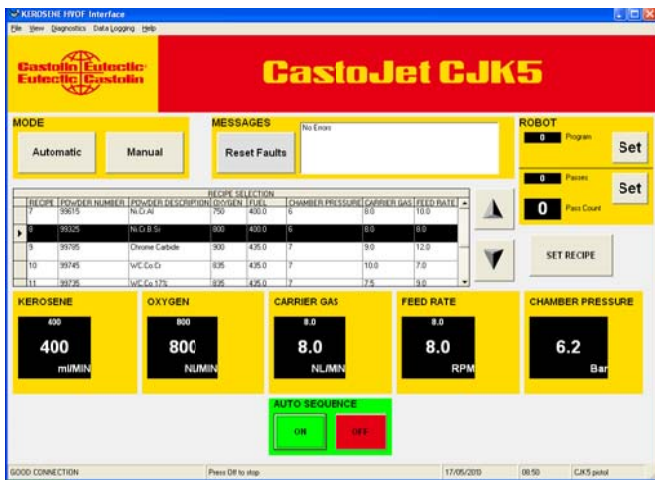
Figure 2: CJK5 touch screen control panel, for monitoring and storage of all parameters during spraying
