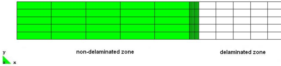
Figure 1: typical 2D-mesh of a test specimen
