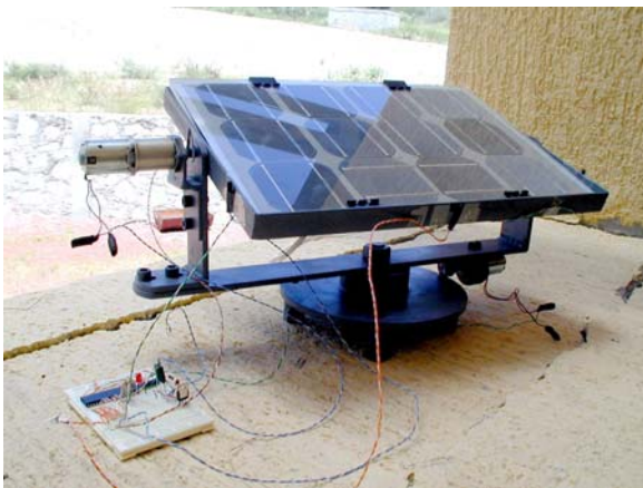
Fig. 3: Automatic two-axis Sun tracking system.
