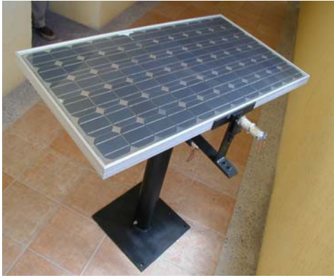
Fig. 3. Photo of solar tracking system
