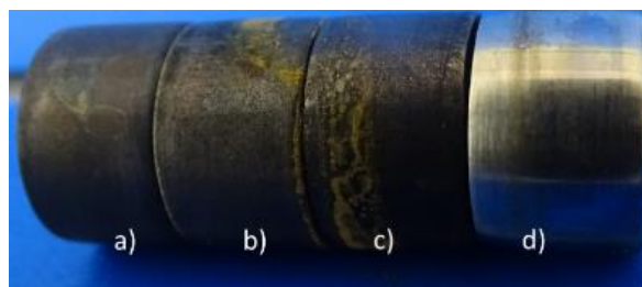
Fig. 5. API 5L X60 iron Working electrodes exposed to a system consisting of: \text{NH}_3=500 ppm, \text{pH}=8.5 (adjusted with \text{H}_2\text{S} ), \text{CN}^- =250 ppm, and T=40^\circ\text{C} , v = 1 mV/s a) Blank ,b)5, c) 25, d)50 ppm of inhibitor DMI.
