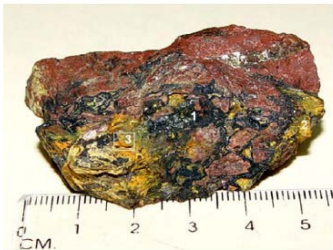
Fig. 3 Photograph of Victorino sample SMV-8, which consists of brecciated ignimbrite. Fragments are set in a matrix made up of (1) black uraninite (2) yellow uranophane and (3) becquerelite (in the white frame)
