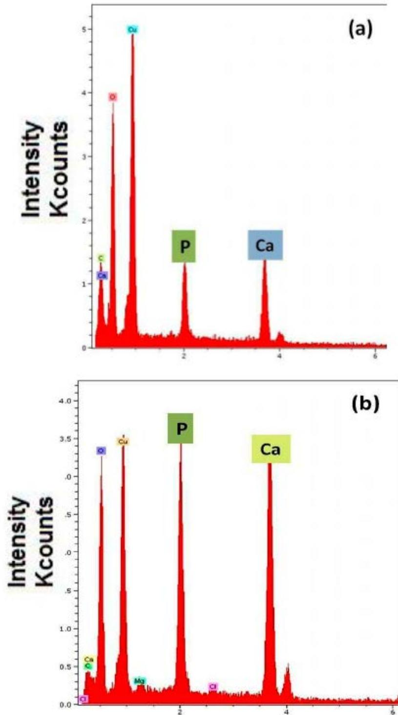
Figure 11. EDS before (a) and after (b) immersion in SBF HA40 composite.
