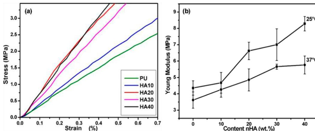
Figure 2. Representative stress–strain curves for PU and PU/nHA composites and Young's module as a function of the content nHA.
