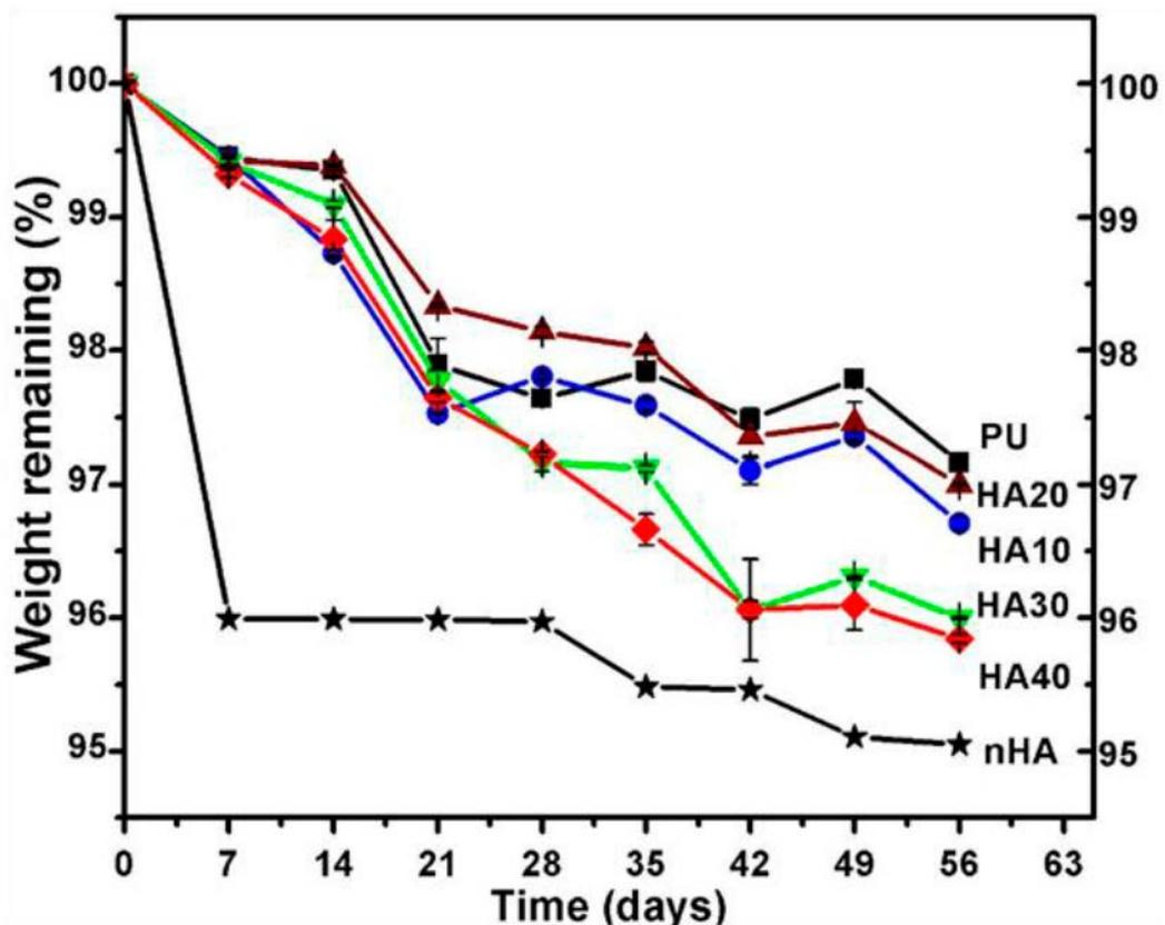
Figure 3. Incubation time of PU and composites in PBS solution versus weight remaining.
