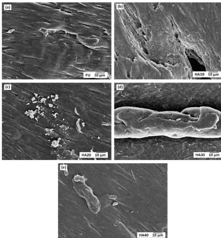
**Figure 1.** Secondary electron images (SEI) of PU and composites before analysis.
