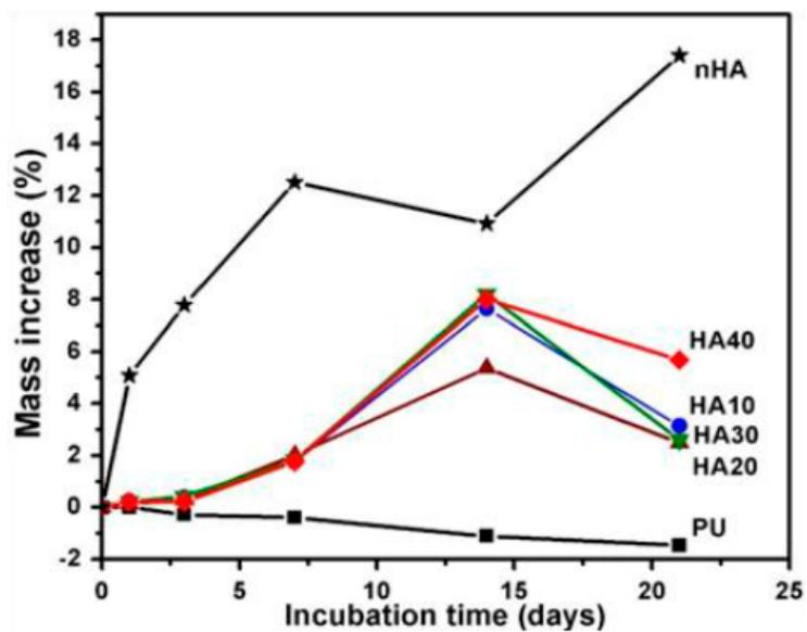
Figure 5. Mass increases of nHA and composites due to incubation time in SBF.
