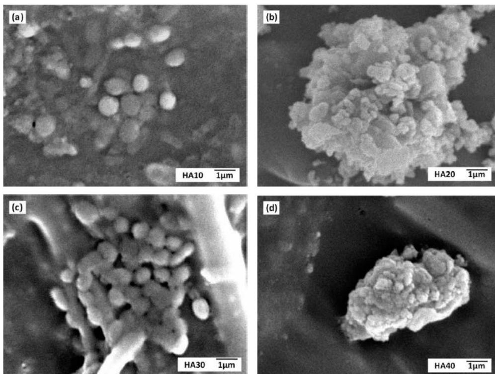
Figure 7. SEM micrographs of composites PU/nHA post-immersion during one day in SBF.
