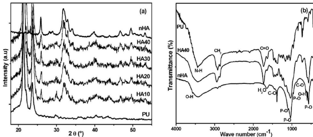
Figure 6. XRD pattern and FT-IR spectra of PU, nHA and composites immersed in SBF for 7 days.
