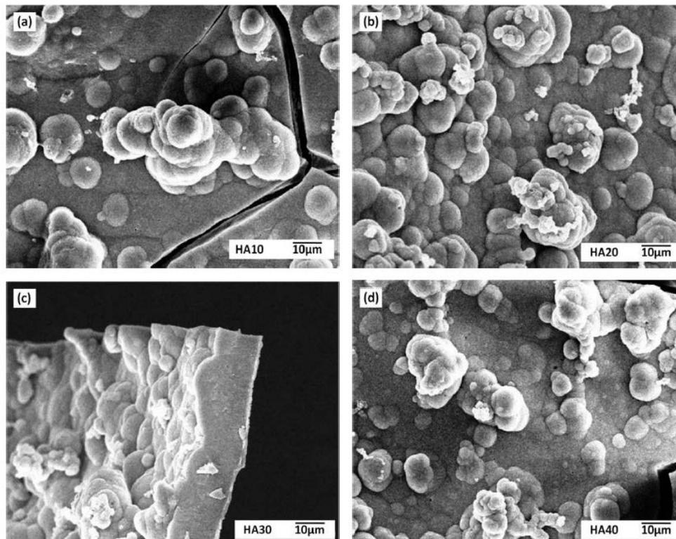
Figure 10. SEM micrographs of PU/nHA composites post-immersion to 21 days in SBF.
