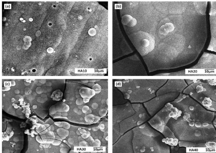
Figure 9. SEM micrographs of PU/nHA composites post-immersion to 14 days in SBF.
