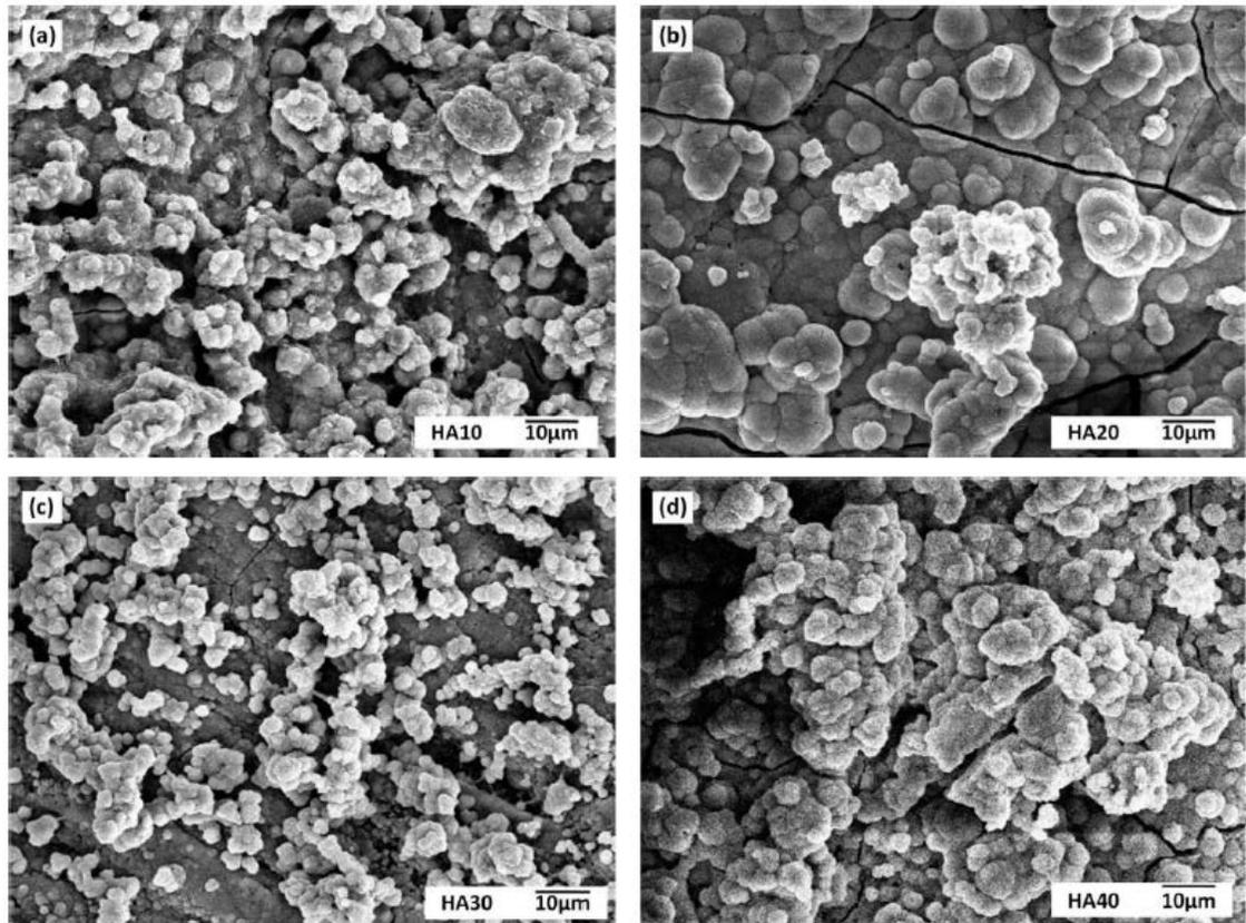
Figure 8. SEM micrographs of PU/nHA composites post-immersion to 7 days in SBF.
