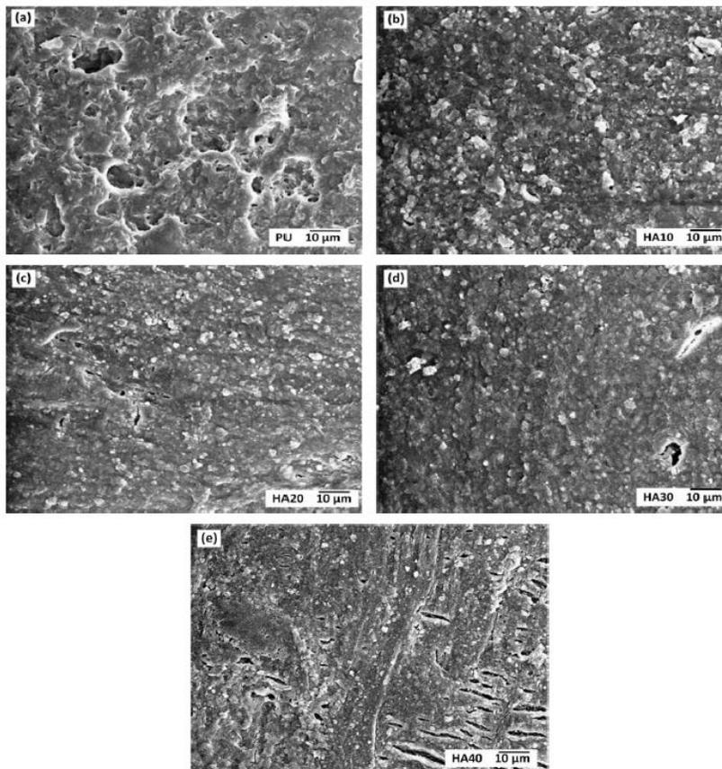
Figure 4. Images by SEM of surface composites post-immersion for 8 weeks in PBS: PU, 10, 20, 30 and 40 HA.
