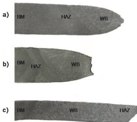
Fig. 4. Optical macrographs of the longitudinal sections (X70 steel) of the specimens after cracked, showing the zone where they failed: (a) tested in air, (b) tested in NACE solution at 25°C and (c) tested in NACE solution at 50°C
