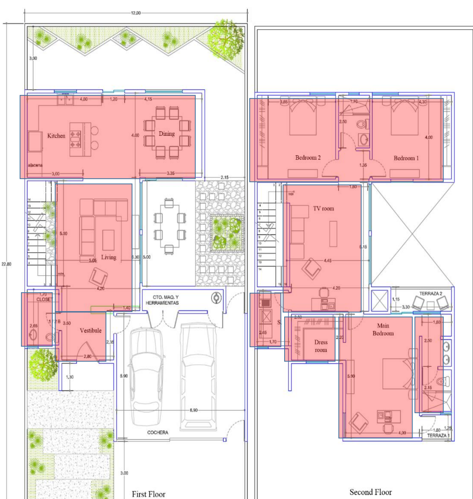
Fig. 2. Radiant floor heating surfaces
