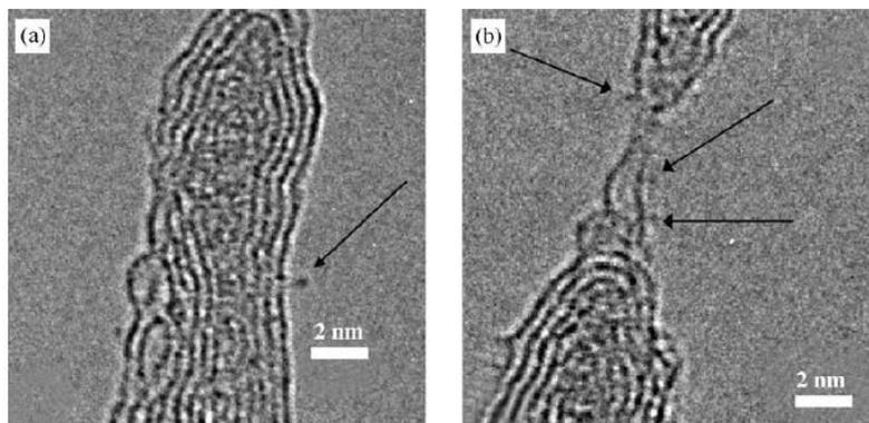
Fig. 4. TEM images of ad-strips. (a) Ad-strip (signalled by arrow) on the surface of graphitic bridge diffusing rapidly during the healing process. (b) Numerous ad-strips (signalled by arrows) returning to CNT neck during the healing process.
