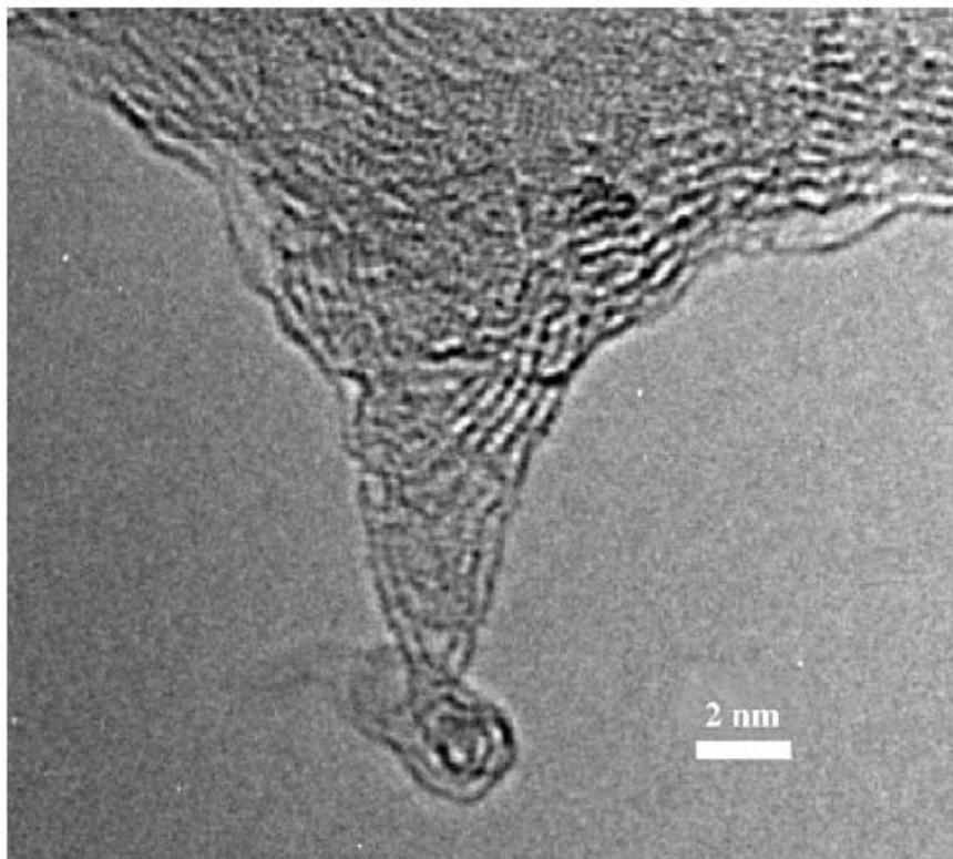
Fig. 3. TEM images of one side of a bridge that has fractured and bent into the beam, so as to be parallel to the beam direction and thereby provide a cross-sectional view of the bridge structure. The cross-sectional view clearly indicates that the bridge neck consists of a CNT that itself necks into some smaller structure, possibly a CNT of smaller diameter.
