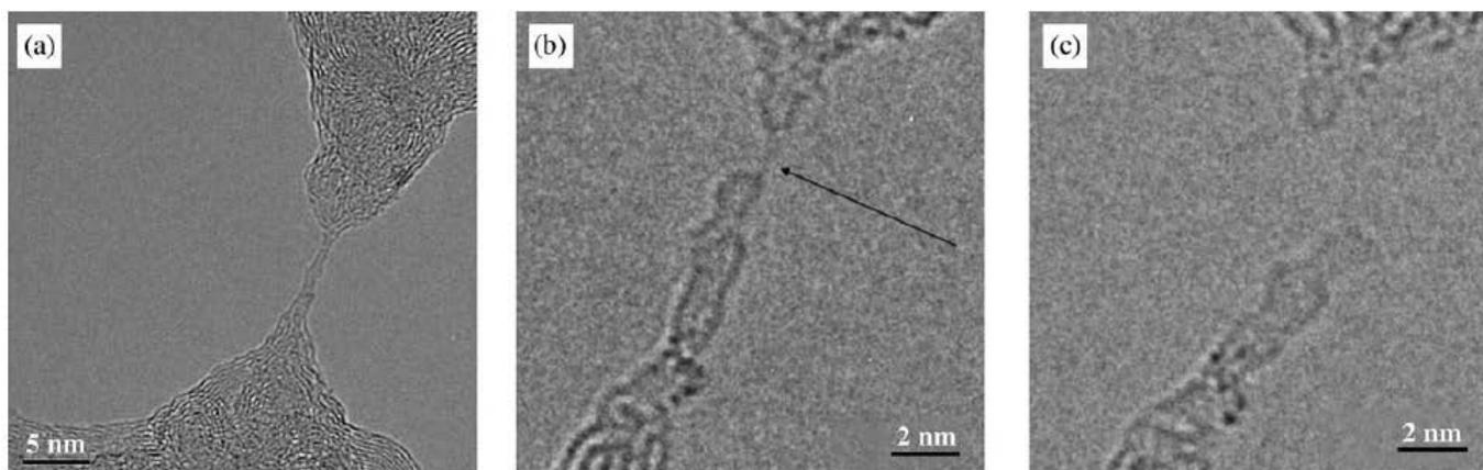
Fig. 2. Sequence of TEM images depicting plastic fracture. (a) A SWCNT is formed in the neck region of the graphitic bridge separating two holes. (b) The SWCNT deforms in response to axial tension and irradiation damage, forming a single chain of carbon atoms of nearly 1 nm in length that remained stable for 5 min (signalled by arrow). (c) The bridge fractures at the chain of carbon atoms upon increasing the current density.
