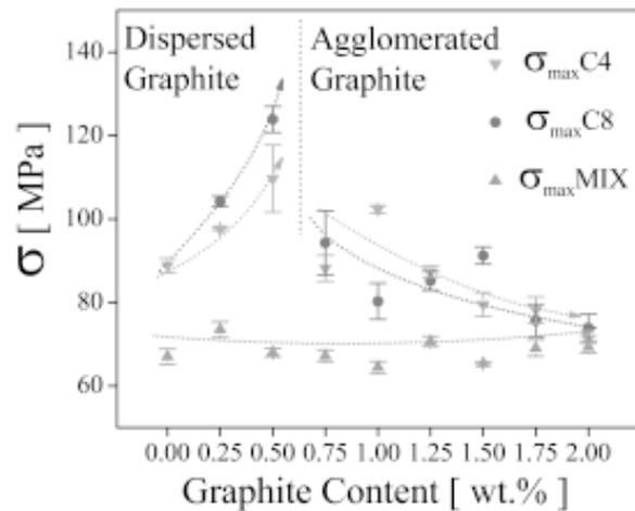
**Fig. 3.** Yield Strength in Al<sub>6063</sub>-C composites. Notice the two regions as a function of graphite content.
