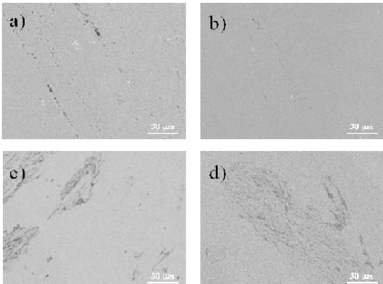
**Fig. 2.** Microstructure in extruded samples, (a)-(b) 0.5 wt.% C, and (c)-(d) 2.0 wt.% C.
