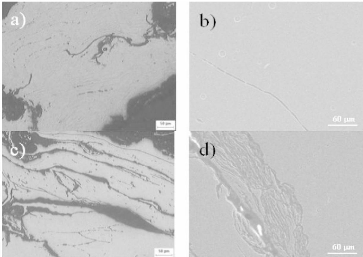
**Fig. 1.** Microstructure observed in as-milled powders; (a)-b) 0.5 wt.% C, and (c)-(d) 2.0 wt.% C.
