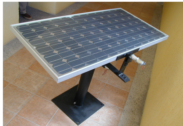
Fig. 4. 2-axis solar tracking PVC, non-concentrated radiation
