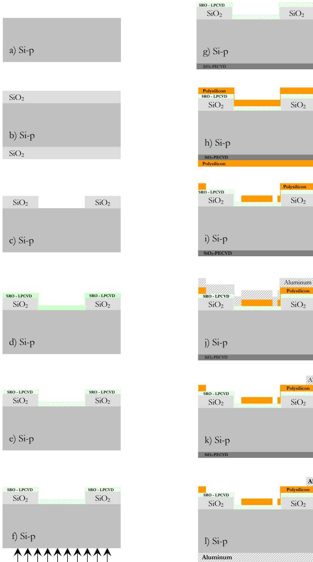
Figure 4.1. Fabrication steps of MOS-like structures.
