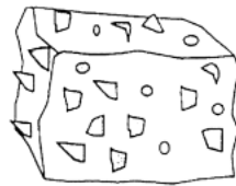
Figure 3. Illustration of a composite material reinforced with particles [3].
