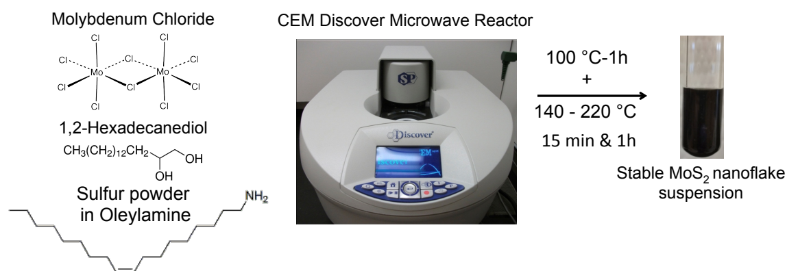
Fig. 8.5. Schematic of microwave synthesis of MoS 2 nanoflakes.
