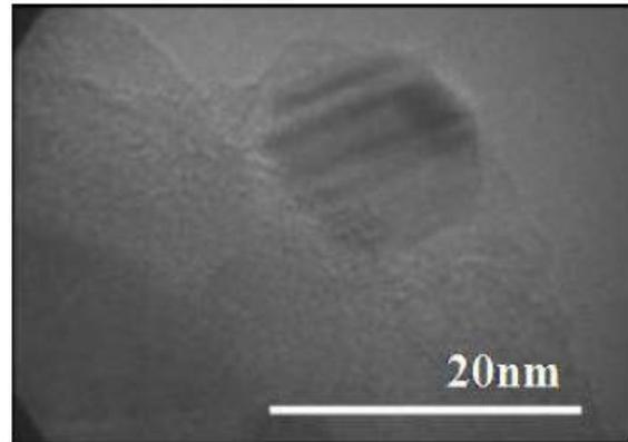
Fig.3. TEM image from Ag-C NP dispersed into Al<sub>2024</sub> alloy.
