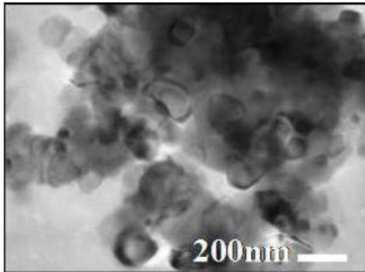
Fig. 1. TEM bright field image of an Al-based composite, showing the crystal size.
