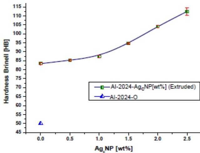
Fig. 5. Brinell hardness as a function of Ag-C NP content.
