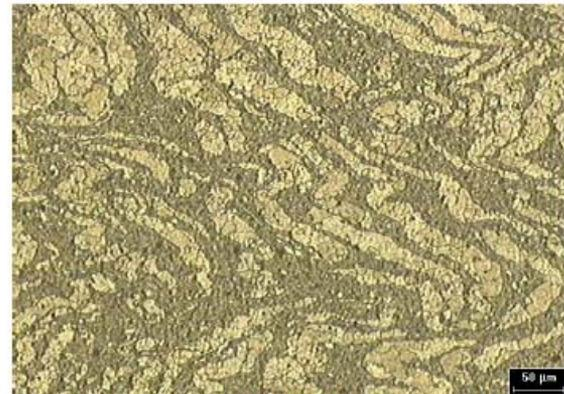
Fig. 4. Optical micrographs of Al<sub>2024</sub> 1.0 wt % in as-extruded condition.
