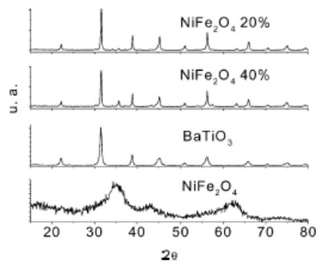
**Figure 1.** Room temperature x-ray diffraction patterns for the cobalt ferrite and barium titanate starting phase, as well as for the composites with 20 and 40 wt.% of nickel ferrite.
