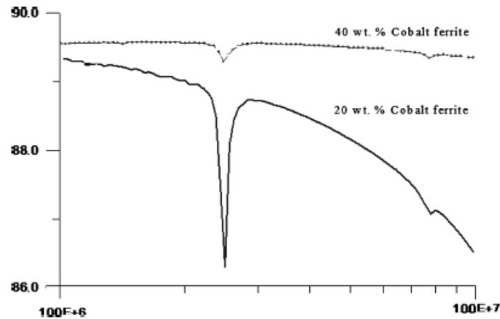
*Figure 4.* Piezoelectric resonance at thickness mode.
