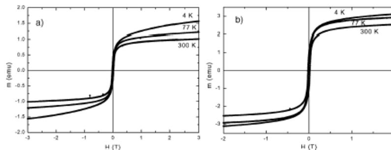
**Figure 2.** Magnetization curves for three different temperatures for the a) 20 wt.% nickel ferrite composite and for the b) 40 wt.% nickel ferrite composite.
