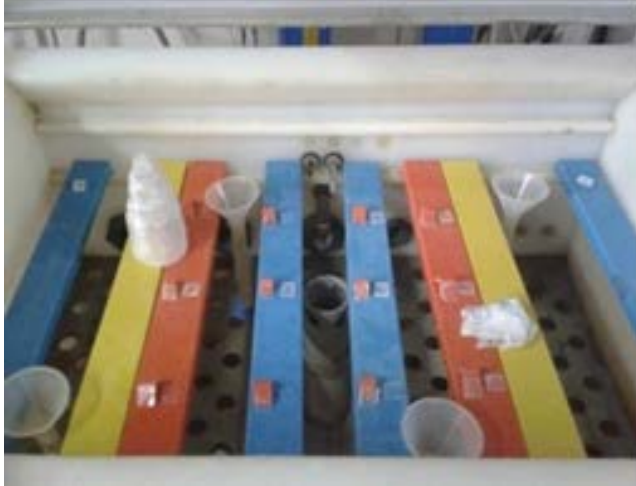
FIGURE 1. Arrangement of gypsum samples inside the climatic chamber.
