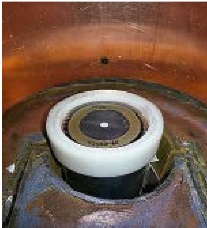
FIGURE 8. ^{60}\text{Co} standard source being measured on the window of a CANBERRA™ XtRa HPGe detector.
