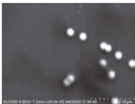
Figure 4: SEM micrograph of synthesized microspheres containing 39% molar amount of IOA (Rx-66, entry 4 of Table 1).
