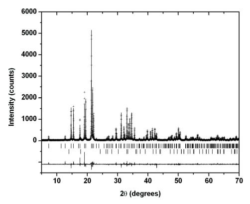
Figure 1 Rietveld refinement for OAp employing synchrotron radiation data. Observed (crosses), calculated (solid line) and difference (bottom trace) plots are represented. Vertical marks correspond to the allowed Bragg reflections for OAp (first row) and  $SiO_2$  (second row).
