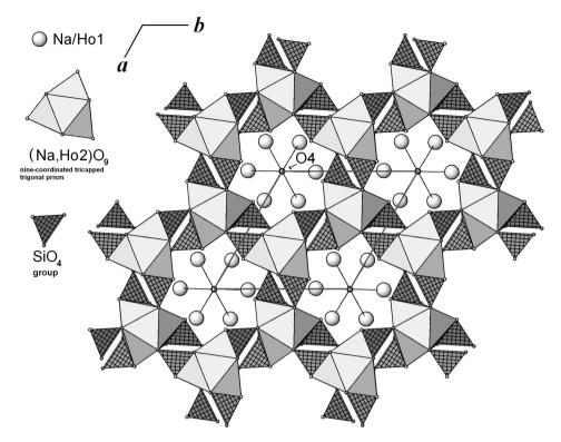
Figure 2 Structural representation of Na<sub>2.27</sub>Ho<sub>7.73</sub>(SiO<sub>4</sub>)<sub>6</sub>O<sub>0.72</sub>.
