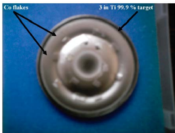
Fig. 1. Titanium target (3 in.) with Co wafers/flakes they were pasted with silver paint.
