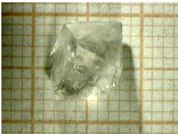
Fig. 1. Picture of a single crystal of the p-LASN.
