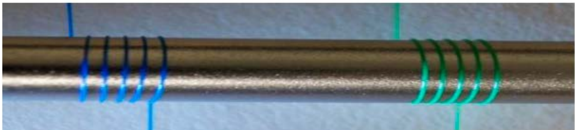
Figure1. Experimental set up. a) Optical fibers rolled up in a steel cylinder.
